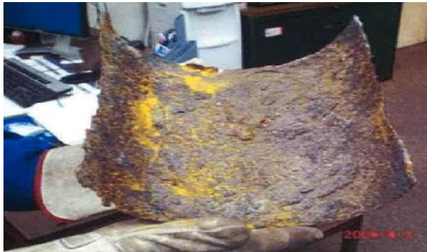
Welded Metallic Saddle Corrosion
