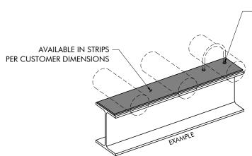
**HOLES IN FLAT PADS** FOR U-BOLTS CAN BE PRE-DRILLED OR LOCATED AND DRILLED AT THE TIME OF INSTALLATION.
